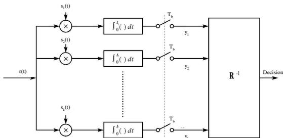
Figure 1: The decorrelating detector structure.
