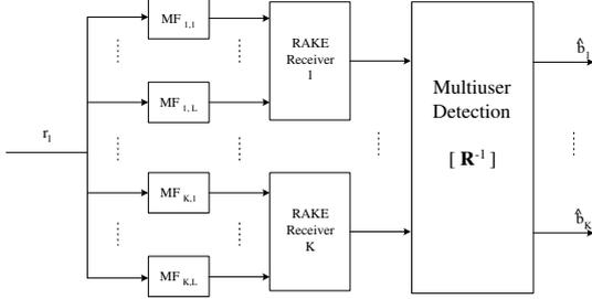
Figure 2: Diagram of a  $L$ -path CDMA system with a decorrelating detector.
